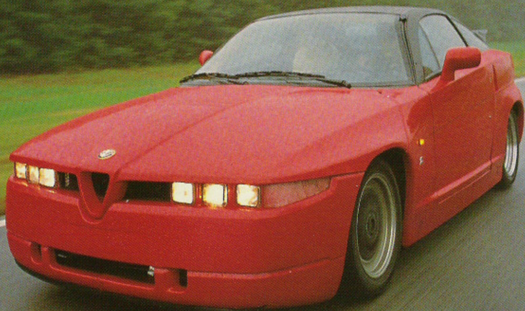
Six Carello lights break large frontal area. Commendable cd is 0.3
